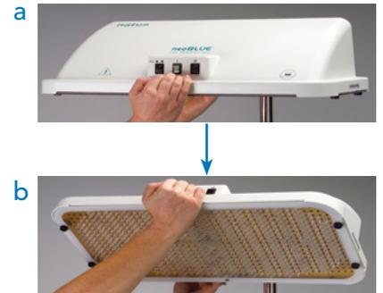
When adjusting the proximity, hold up the neoBLUE light enclosure with one hand to lessen the weight on the rail.
