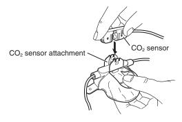
6. Perform zero calibration. For details about zero calibration, refer to the operator's manual of the connected monitor.
